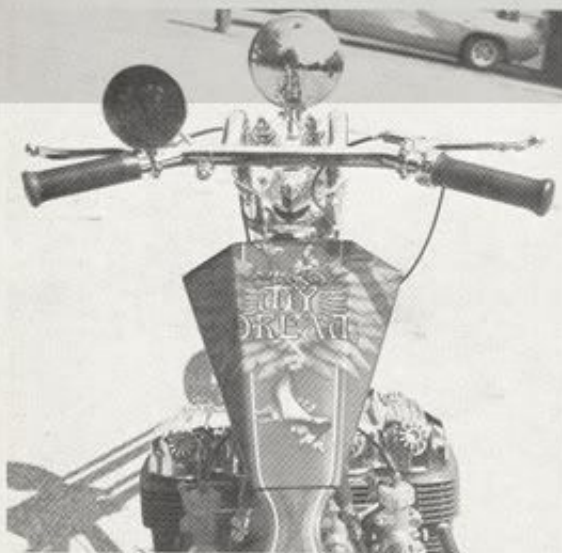
ABOVE — Molded removable tank and paint work are once again from Denvers. Drag style bars fit inside springer legs.
